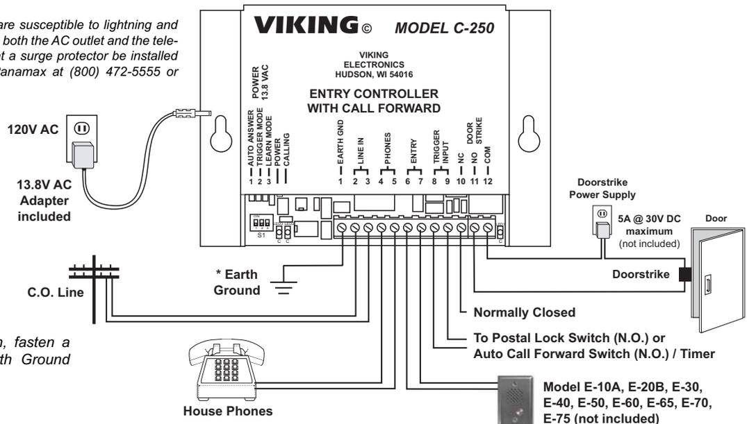
\* **Note:** To increase surge protection, fasten a wire from the screw terminal to Earth Ground (grounding rod, water pipe, etc.)
