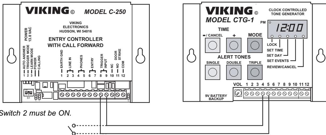
Note: DIP Switch 2 must be ON.
